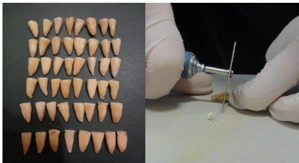
Figure 1. Samples after cutting the tooth crown using diamond disk
