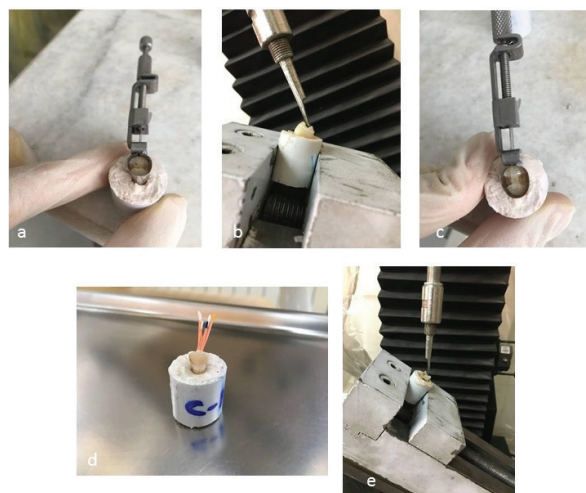
Figure 1. a) Prepared tooth ready for restoration b) Tooth under load c) ribbon fiber placement d) RCT-Obturation e) Tooth fracture at the end of test
