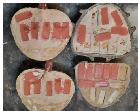
Figure 1. Muffled acrylic blocks. The right side is the flexible acrylic blocks and the left side is the heat-cure blockes
